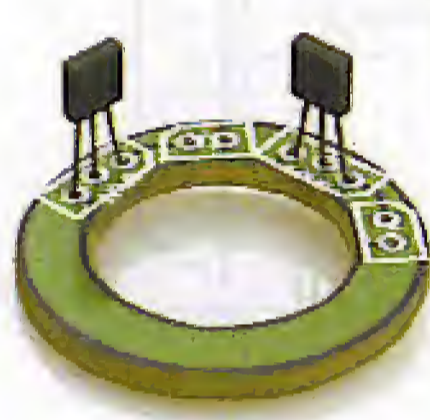
Figure 4. Component mounting plan on the elongated PCB. The small section is intended for the two Hall sensors.
