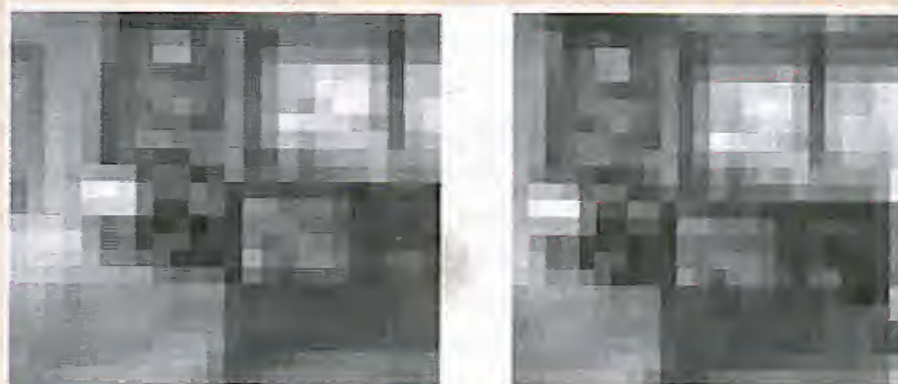
Figure 3. These are two images recorded by the sensor 0.67 ms apart. From this information the DSP calculates the displacement in the X- and Y-direction. (source: Agilent)
