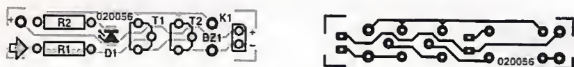
Figure 1. The narrow board and the two miniature batteries together fit into a metal tube to make a probe-like enclosure for the tester.
