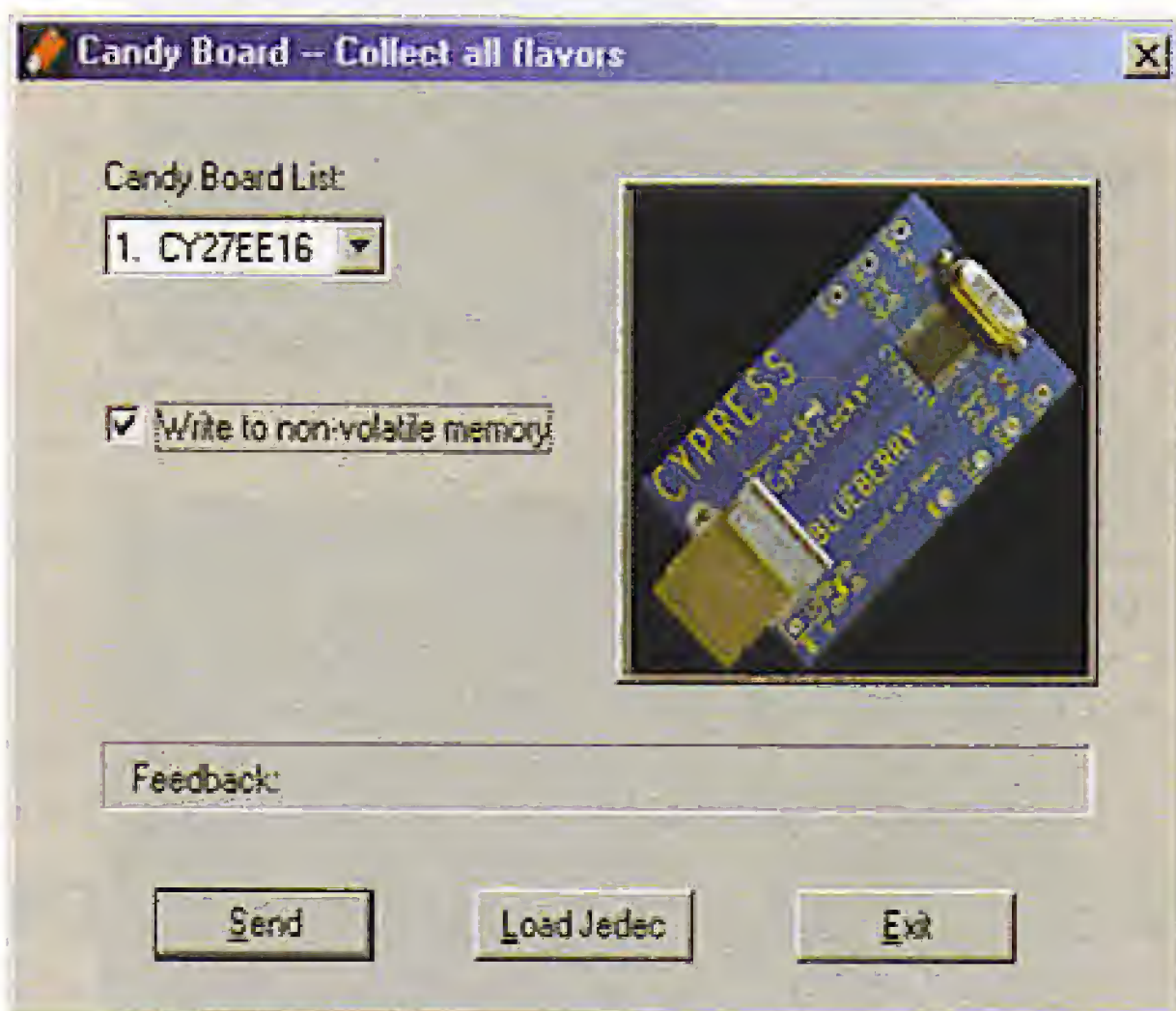
Figure 7. Programming the settings into EEPROM.
