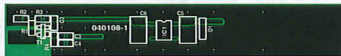
Figure 2. The PCB has been designed with compactness and low input capacitance in mind — hence the use of SMD parts.
