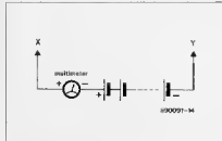
Fig. 4. Auxiliary circuit for adjusting the PSU.
