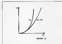
Fig. 3. Current vs. applied voltage characteristic in the forward bias region with and without the effect of bulk resistance.
