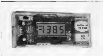
This compact, ICL7126-based LC display unit can be used in many applications.
