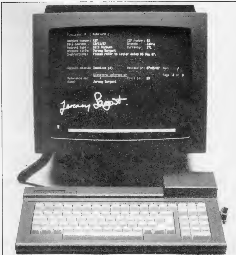
The j300 enables graphics to be shown together with file data — a possible extension to a criminal records facility.
