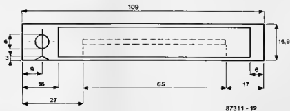
Fig. 3. Cutting and drilling details for the music cassette box.
