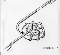
Fig. 10. Interference from the computer can be suppressed by winding the serial data and supply cables onto a ferrite core.
