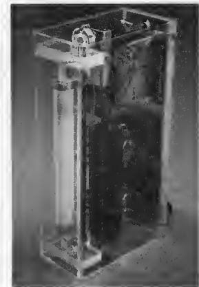
Figure 4: The power transistors and the transformer are not mounted on the PCB. All other components can be accommodated on a small SELEX PCB of size 1.
