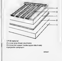
Fig. 7. Alternative construction of a paperholder, which is essentially a PCB sandwich. The HV electrode is formed by the un-etched copper surface on the lower circuit board. The upper electrode is earthed.
