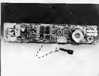
Fig. 12. Completed HF controller ready for fitting into the tube armature.
