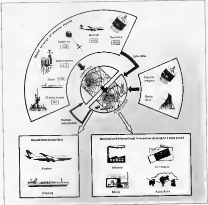
Steps from observation to forecast. Numbers indicate the average number of observations each day for use in the main 0000 utc and 1200 utc global numerical forecast model runs.
