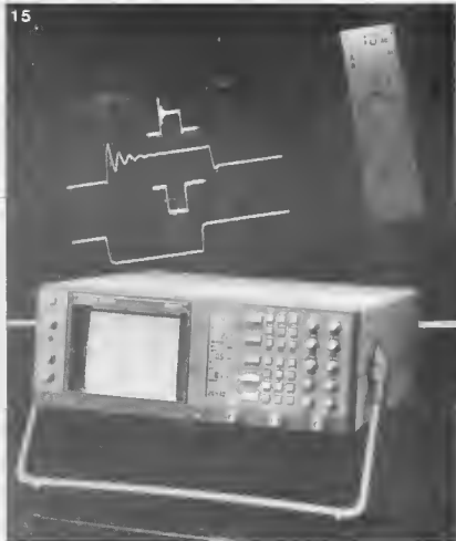
Fig. 15. Front view of the PM3050 with the trace and LCD shown enlarged
