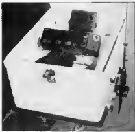
Motorcycle top box with Storno's "Silent Messenger" radio installed in a shock absorbent enclosure.
