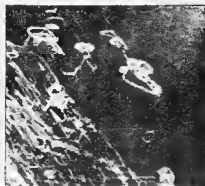
Three topographs from a sequence showing the movement and multiplication of dislocations during the plastic deformation of a single crystal of ice at -20^{\circ}\text{C} . These illustrations are negative prints, so dislocations appear bright against a dark background. The width of the region shown is 4 mm on the crystal.
