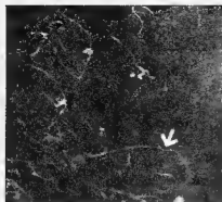
Three topographs from a sequence showing the movement and multiplication of dislocations during the plastic deformation of a single crystal of ice at -20^{\circ}\text{C} . These illustrations are negative prints, so dislocations appear bright against a dark background. The width of the region shown is 4 mm on the crystal.
