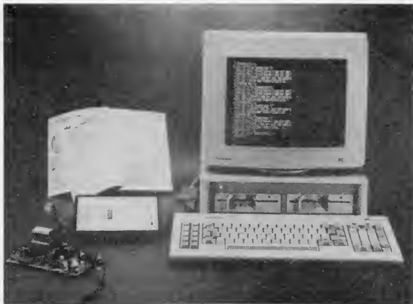
Fig. 9. A prototype of the EPROM emulator used in conjunction with an Amstrad PC1512 host computer.
