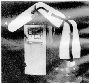
The RDP anthropomorphic robot with trunk, shoulder, elbow and wrist joints, enables loads up to 35 kg to be manoeuvred "over the shoulder".
