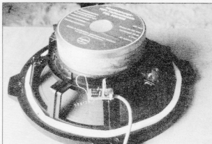
Fig. 7. The modified bass drive unit: note how the impedance changer is fixed to its chassis.
