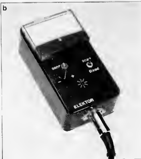
Fig. 23. Circuit diagram (23a) and practical outlook (23b) of the aerial positioning unit
