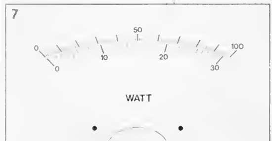
Fig 7 Suggested scale divisions to match the meter's range factor of \frac{1}{10} ( \approx 3.16 ).
