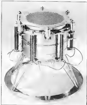
The UK 10-centimetre diameter ion thruster, designed for station-keeping of multi-tonne communications satellites, now being tested with xenon propellant.
