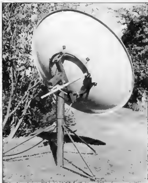
Fig. 2. Rear view of a dish, fitted with the Polar Mount satellite tracking system which enables easy dish positioning for satellites at different orbital positions (Photograph reproduced here by courtesy of Harrison Electronics)
