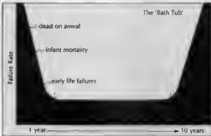
The so called bath tub curve that relates operating time and failure rate
