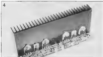
Fig. 4 Completed assembly of PCB and heat sink
