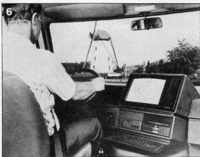
Fig. 6. CARIN in action. The keyboard will in future be replaced by a touch screen. (Philips Press Photograph)
