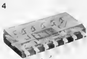
Fig. 4. Already there is ample choice of surface-mount ICs. Shown here is a typical example in a SO-14 package.
