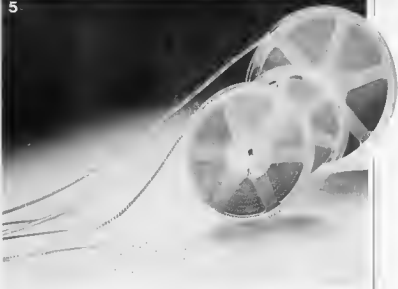
Fig. 5. For mass production, SMDs are delivered in blister tape, i.e. a series of compartments separated by a thin polythene tape. The tape can be fed into automatic mounting equipment. SMDs are, however, also available in different packing
