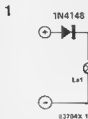
Figure 1. The lamp glows if the polarity of the test voltage is correct.
