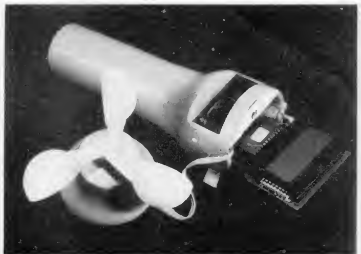
Fig. 5 Suggested construction of the sensor and the carrier for the set of cups (scale=13:20).
