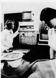
Harwell developed ultrasonic inspection system in use at Moorfields Eye Hospital, London displays ultrasonic images of the eye directly on a television screen and allows them to be recorded on a standard video recorder.
