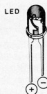
Figure 5. Increasing the resistance reduces the current, thus reducing the glow of the LED.
