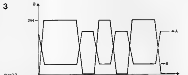
P 1 . The setting of P 1 is optimum when the voltage at its wiper (wave form A in figure 3) is exactly opposing the input voltage (wave form B in figure 3).
