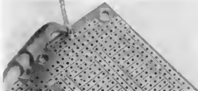
Figure 10 Working with solder sucking stranded wire.
