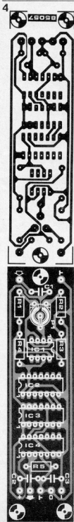
Figure 4. The printed circuit board of the generator is small enough to be built into an existing sine wave or function generator.
