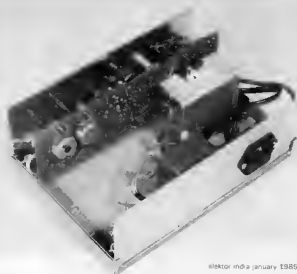
Figure 7. In this photo the function generator is completely finished, except for the lid which still has to be put on the case. The mains cable travels via the printed circuit board to the power switch on the front panel. Both voltage regulators (on the reverse side of the board) are fixed onto a home-made heatsink. The wire-wound potentiometer for the frequency setting is located under the heatsink.
