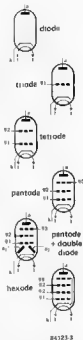
Figure 3. These are the graphical symbols used to depict some of the most common types of valve.
