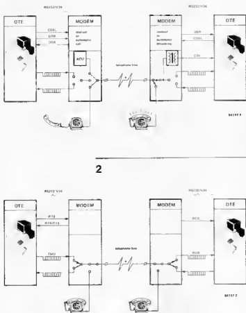
Figure 1. This is the procedure for a call, whether it is manual (when the user dials the number) or automatic (ACU). The ringing is detected by the receiving modem, which then signals the DTE by activating the CIN line.
