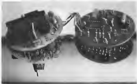
Photo 1 Here we see the two boards that make up the tachometer. To achieve the compact form shown in the photo at the beginning of this article the two are mounted one above the other in the form of a 'sandwich'.
