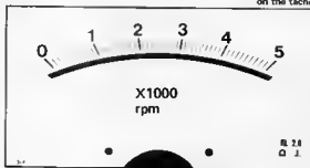
Figure 2b. This is a suitable scale to use for the meter on the tachometer.
