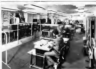
IRAS control centre at RAL, responsible for monitoring the status of the satellite and collecting data from its primary telescope and other experiments. The satellite passes over the centre at least twice daily. Incoming data gives scientists a brief check on objects that have been observed and controllers can make checks on the spacecraft itself. Data is sent to the Jet Propulsion Laboratory for complete processing.
