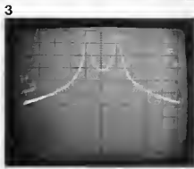
Figure 3. Frequency spectrum of a carrier frequency-modulated by a square wave of 10 Hz at a deviation of 100 Hz.
