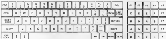
Figure 3. This shows the actual mounting positions of the keys in the keyboard.
