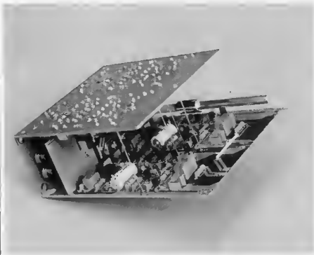
Photo. The complete MC/MM phono preamp module. Once all the connecting wires are in position, it is a fairly rigid construction.
