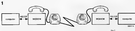
Figure 1. The use of a modem is illustrated in this drawing. Each modem can act as either a transmitter or as a receiver.
