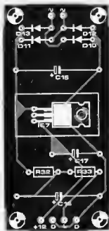
Figure 5. The printed circuit board for the power supply. Only one is required.
