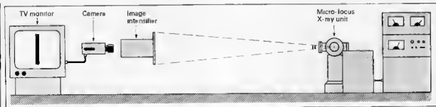
Typical direct-viewing X ray system incorporating a particulate phosphor, which converts X-ray photons to electrons of similar spatial distribution. A high voltage accelerates the electrons to a smaller, output phosphor, where the image formed can be viewed directly using an optical device or a television camera.
