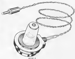
Figure 3. The construction of the matchbox radio is illustrated here. The 'chassis' is made from plastic sheet and fits inside a matchbox. There is plenty of room for all the components including the output stage if required.
