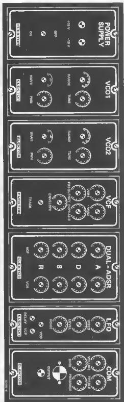
Figure 9. A suggested front panel layout for the various modules.
