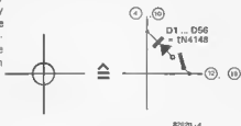
Figure 4. Every junction in the matrix shown in figure 3 consists of a diode and a key
