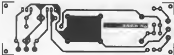
Figure 9. The power supply board for the circuit in figure 7. The wire link situated next to D4 provides the connection for the unbalanced -23.5 V voltage.
