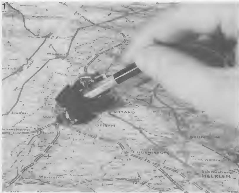
Photo 1. An alternative solution towards constructing the sensor. This does not operate on the light interruption principle, but uses the light reflected by the black-and-white squares. That is why this particular sensor must be 'light-proof'.
