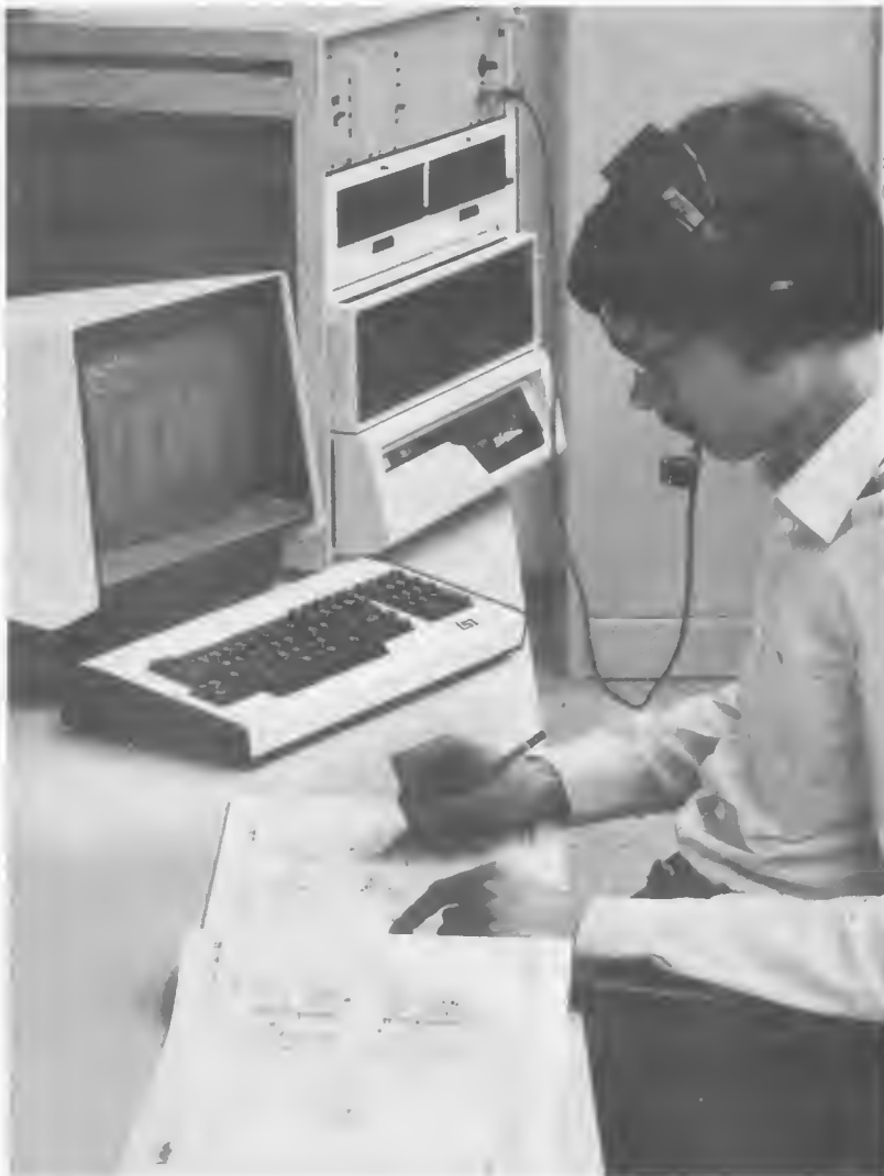
Photo. The acoustic data reception system (ADES) by AEG-Telefunken is being used here to produce wiring diagrams. The operator can enter the data from the circuit diagram directly into the computer by means of a microphone. Afterwards, the computer has to 'read back' the data display via the headphones, so that any mistakes can be corrected. (Photo by AEG-Telefunken.)
