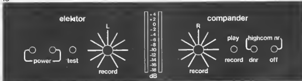
Figure 15. The front panel design for the Elektor High Com system. It is not shown in full size.
