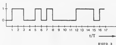
Figure 3. This shows a brief portion of the output from the random sequence generator.
