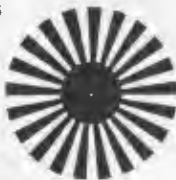
Figure 5. The segmented disc can be cut out and glued onto a circular piece of perspex.
