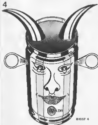
Figure 4. The LEDs and the LDR should be positioned so that they face the 'marksman'.
