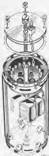
Figure 2. The side view of the inside of the bath thermometer shows the principle components involved in the construction.
