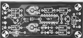
Figure 3. Component overlay and track pattern of the printed circuit board for the fridge alarm.
